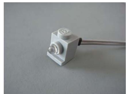
Figure 5. Fitting a LifeLite in a headlight brick.
