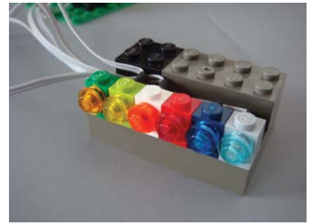
Figure 2. Lifelites installed inside headlight bricks.
